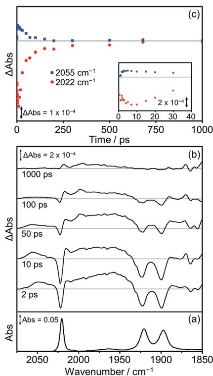
Fig. 10 FTIR and TRIR spectra of **Dyad 1 Br** in THF: (a) FTIR ground state spectrum; (b) TRIR difference spectra taken at 2, 10, 50, 100 and 1000 ps after flash photolysis at 560 nm; (c) TRIR single point kinetic traces for the depletion and reformation of the ground state bands (red dots, 2022  $\text{cm}^{-1}$ ) and the growth and decay of the <sup>3</sup>MLCT excited state (blue squares, 2055  $\text{cm}^{-1}$ ). Inset shows expansion of the first 40 ps.
