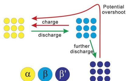
Fig. 3 Schematic diagram of phase transitions in Al-doped  $\text{Li}_4\text{Ti}_5\text{O}_{12}$  under different discharging cutoffs, in which  $\alpha$  is the delithiated phase,  $\beta$  is the lithiated phase, and  $\beta'$  is the lithiated phase discharged to a very low cutoff potential.
