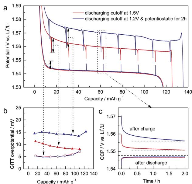
Fig. 2 (a) GITT measurements for Al-doped Li<sub>4</sub>Ti<sub>5</sub>O<sub>12</sub> (ALTO), which consist of a series of current pulses applied at 0.1 C for 1 h, each followed by a 2 h relaxation period. The charging cutoff is 2.0 V, and the discharging cutoffs were 1.5 V (red) and 1.2 V and potentiostatic for 2 h (blue). (b) Potential increments (decrements) and (c) OCPs during the relaxation periods.
