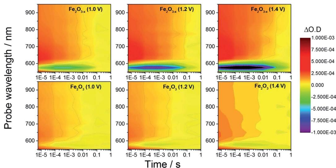
Fig. 2 TA spectra of  $\alpha$ -Fe<sub>2</sub>O<sub>3</sub> and  $\alpha$ -Fe<sub>2</sub>O<sub>3-x</sub> at various applied potentials (vs. RHE) in 1 M NaOH with the photoanodes excited from the electrolyte/electrode side (EE) with a 355 nm (6 ns pulse) laser.
