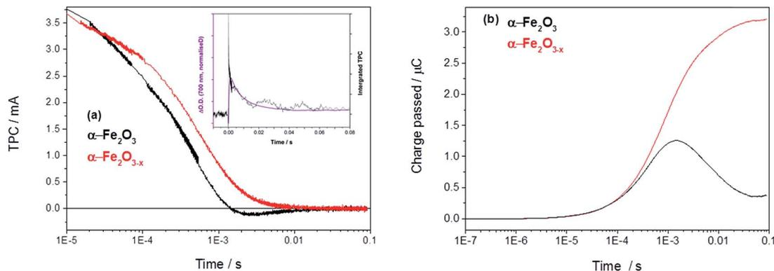
Fig. 4 (a) TPC decays of  $\alpha\text{-Fe}_2\text{O}_3$  and  $\alpha\text{-Fe}_2\text{O}_{3-x}$  held at  $1.4 V_{\text{RHE}}$  with an inset showing the overlay of the decay of the TA with the integrated TPC in  $\text{Fe}_2\text{O}_3$  at  $1.4 V_{\text{RHE}}$  (Fig. S6†) and (b) the converted total charge passed following UV excitation (355 nm, 6 ns).
