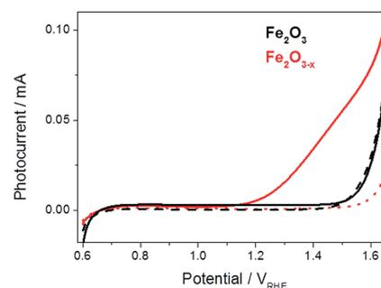
Fig. 1 Linear sweep voltammograms for  $\alpha$ -Fe<sub>2</sub>O<sub>3</sub> (black) and  $\alpha$ -Fe<sub>2</sub>O<sub>3-x</sub> (red), 5 mV s<sup>-1</sup>, under low power white light illumination (solid line, *ca.* 0.1 sun) and in the dark (dashed line).
