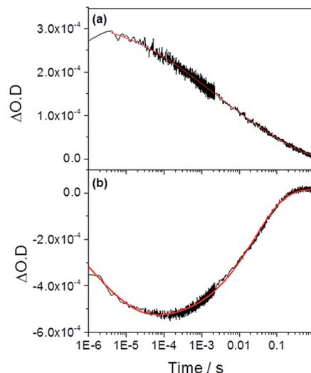
Fig. 6 TA traces recorded at (a) 700 nm (photoholes) and (b) 580 nm (electron trap state) in  $\alpha$ -Fe<sub>2</sub>O<sub>3-x</sub> at 1.4 V<sub>RHE</sub> following UV excitation (355 nm) in 1 M NaOH. The red lines correspond to the fitted functions identified in the main text. Full parameters can be found in the ESI.†
