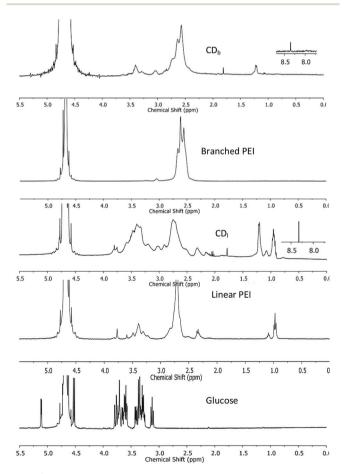
Fig. 2  $\,^{1}$ H NMR spectra of CDs passivated with branched PEI (CD<sub>b</sub>) and linear PEI (CD<sub>l</sub>), control spectra obtained from branched and linear PEI, and glucose.
