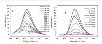
Fig. 4 Excitation-dependent PL emission of the carbon dots passivated with (a) branched PEI ( $CD_b$ ) and (b) linear PEI ( $CD_b$ ).
