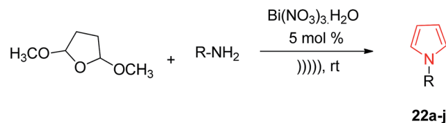
Scheme 4 Synthesis of N -substituted pyrrole derivatives by an eco-friendly route using ultrasound-assisted bismuth nitrate-catalyzed reaction.
