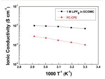
Fig. 4 Temperature-dependent ionic conductivity (temperature range =  $30-70\,^{\circ}$ C) of PC-CPE and carbonate-based liquid electrolyte (1 M LiPF<sub>6</sub> in EC/DMC =  $1/1\,\text{v/v}$ ).
