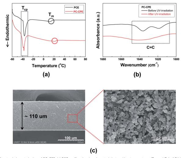
Fig. 1 Structural characterization of PC-CPE: (a) DSC profiles showing characteristic transition temperatures ( $T_{CP}$  and  $T_{m}$ ) of SN in PCE and PC-CPE; (b) FT-IR spectra (before/after UV curing) of acrylic C=C bonds of ETPTA in PC-CPE; (c) cross-sectional FE-SEM images of PC-CPE, wherein the high-magnification view exhibits the presence of well-reticulated interstitial voids (originally occupied with PCE) formed between the Al<sub>2</sub>O<sub>3</sub> nanoparticles.
