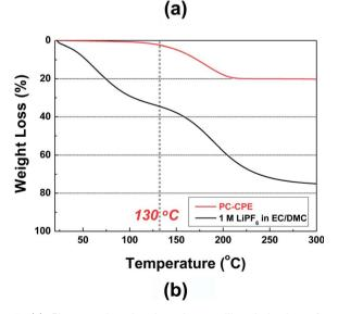
Fig. 7 (a) Photographs showing the swelling behavior of cells assembled with PC-CPE or carbonate-based liquid electrolyte (1 M LiPF<sub>6</sub> in EC/DMC = 1/1 v/v), after exposure to thermal shock (=130 °C/0.5 h). (b) Dynamic mode TGA profiles of PC-CPE and carbonate-based electrolyte (1 M LiPF<sub>6</sub> in EC/DMC = 1/1 v/v).
