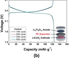
Fig. 5 Charge/discharge profiles of coin-type full cells as a function of cycle number, wherein the cells are cycled at a constant charge/discharge current density of 0.2 C (=0.40 mA cm $^{-2}$ )/0.2 C under a voltage range of 1.5–2.7 V: (a) LiCoO $_2$ /PC-CPE/Li $_4$ Ti $_5$ O $_{12}$ ; (b) LiCoO $_2$ /PE separator/Li $_4$ Ti $_5$ O $_{12}$ .
