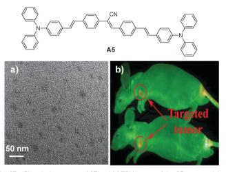
Fig. 17 Chemical structure of A5 and (a) TEM image of the A5 nanoparticles and (b) in vivo fluorescence image of mice bearing subcutaneous tumor xenografts upon injection of A5 nanoparticles (top) and RGD-A5 nanoparticles (bottom) (reprinted with permission from ref. 20, Copyright 2011 Elsevier B.V.).
