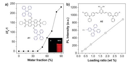
Fig. 15 (a) A typical AIE phenomenon: plot of  $I/I_0 - 1$  as a function of water fraction in THF-water mixtures, where I and  $I_0$  are the fluorescence intensities of A1 in THF-water mixtures in the presence and absence of water, respectively (reprinted with permission from ref. 126, Copyright 2012 Royal Society of Chemistry). (b) Plot of the fluorescence intensity versus the weight ratio of A2 in BSA nanoparticles (reprinted with permission from ref. 127, Copyright 2012 Wiley-VCH)
