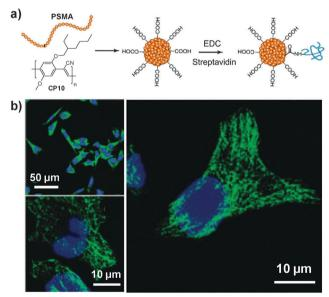
Fig. 9 Chemical structure of CP10. (a) Surface functionalization of CP10 based nanoparticles and subsequent streptavidin bioconjugation via EDCmediated coupling reaction. (b) Confocal images of microtubules in HeLa cells labeled with streptavidin-functionalized CP10 nanoparticles (reprinted with permission from ref. 99, Copyright 2012 Royal Society of Chemistry).
