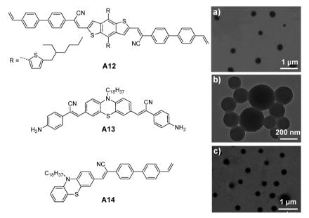
Fig. 24 Chemical structures of A12, A13 and A14. TEM images of (a) A12, (b) A13 and (c) A14 nanoparticles prepared from RAFT, ring-opening polymerization and emulsion polymerization (reprinted with permission from ref. 146-148, Copyright 2013, 2014 and 2014 Royal Society of Chemistry).
