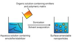
Schematic illustration of the preparation of polymerencapsulated organic nanoparticles from emulsion
