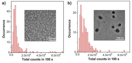
Fig. 14 Histograms of the total number of photons collected for (a) silica-coated F127-PFBT nanoparticles and (b) DSPE-PEG-PFBT nanoparticles.  $\lambda_{\rm ex}$  = 488 nm. Insets show the TEM images of (a) and (b), respectively
