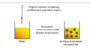
**Scheme 4** Schematic illustration of the preparation of polymer-encapsulated organic nanoparticles from nanoprecipitation.
