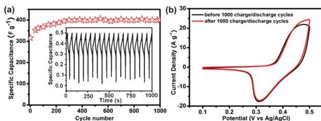
**Fig. 6** (a) The cycle performance of graphene/ZnO hybrid electrode at the current density of  $6.70 \text{ A g}^{-1}$  in  $2.0 \text{ M KOH}$  solution. The inset shows the charge–discharge profile for the graphene/ZnO hybrid electrode. (b) CV of graphene/ZnO hybrid electrode before and after 1000 charge–discharge cycles.
