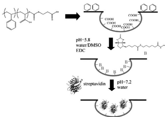
**Fig. 12** Synthetic approach to a streptavidin microarray with immobilization of protein selectively in the pores. Re-printed from E. H. Min, K. H. Wong and M. H. Stenzel, Microwells with patterned proteins by a self-assembly process during honeycomb structured porous films, *Adv. Mater.*, 2008, **20**(18), 3350–3356.
