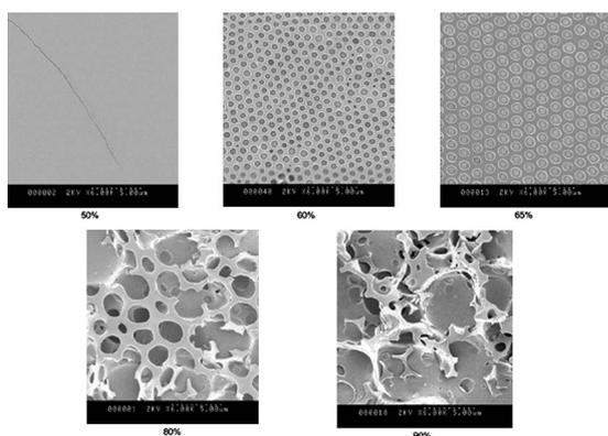
**Fig. 4** SEM images of membranes from PS<sub>75</sub>-*b*-PDMA<sub>30</sub> (10 g L<sup>-1</sup> in 70 : 30 v/v% CS<sub>2</sub>-CH<sub>2</sub>Cl<sub>2</sub>) at constant airflow and different relative humidity values. Re-printed from K. H. Wong, T. P. Davis, C. Barner-Kowollik and M. H. Stenzel, Honeycomb structured porous films from amphiphilic block copolymers prepared *via* RAFT polymerization, *Polymer*, 2007, **48**, 4950–4065.
