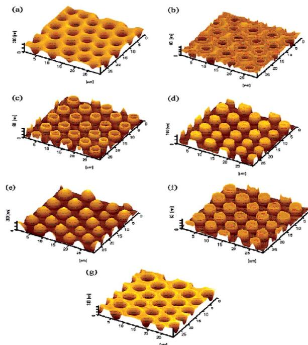
**Fig. 13** AFM images showing the 3D topography of porous films with reversible switchable behaviour when exposed to solvent vapors (a) cast honeycomb film, (b–e) after exposure to CS<sub>2</sub> vapor for 10 min, 15 min, 20 min; and (f–g) after exposure to chloroform for 5 min and 10 min, respectively. Re-printed from L. Cui, Y. Xuan, X. Li, Y. Ding, B. Li and Y. Han, Polymer surfaces with reversibly switchable ordered morphology, *Langmuir*, 2005, **21**, 11696–11703.
