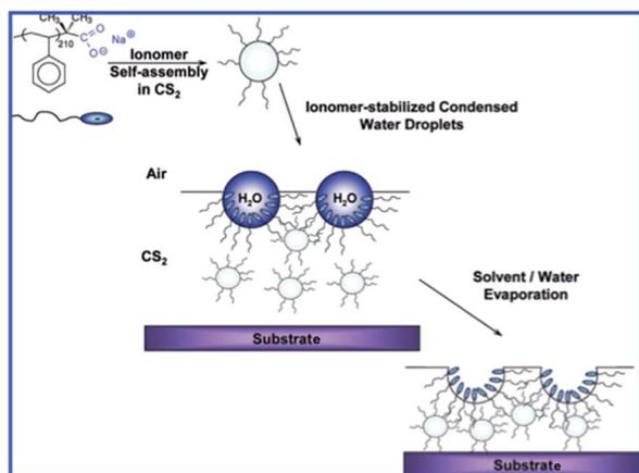
**Fig. 11** Representation of the formation of the honeycomb structured films by ionomer-stabilized condensed water droplets. The pores possess a functionality. Re-printed from L. Billon, M. Manguian, V. Pellerin, M. Joubert, O. Eterradosi and H. Garay, Tailoring highly ordered honeycomb films based on ionomer macromolecules by the bottom-up approach, *Macromolecules*, 2009, **42**, 345–356.
