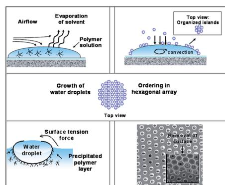
**Fig. 2** Mechanism of formation of honeycomb structured porous polymer films. Adapted from M. H. Stenzel, Formation of regular honeycomb pattern porous film by self-organization, *Australian Journal of Chemistry*, 2003, **55**, 239–243.
