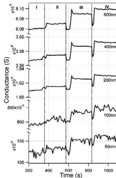
**Fig. 9** Time response of DNA hybridization on five sensors with different dimensions at 4 stages of the experiment. I: DI water; II: 10 nM non-complementary DNA solution; III: 10 pM complementary DNA solution; IV: 100 pM complementary DNA solution. Reproduced from ref. 17 (Li *et al.*, *Appl. Phys. A: Mater. Sci. Process.*, 2005, **80**, 1257–1263) with kind permission of Springer Science and Business Media.
