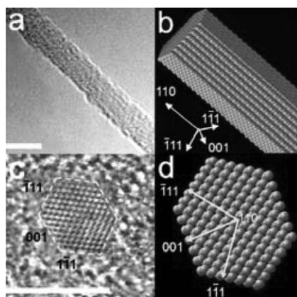
**Fig. 6** (a) 3.8 nm Si-NWs grown along the  $\langle 110 \rangle$  direction, (c) cross-sectional image, and equilibrium shapes for (b) NW and the (d) NW cross-sections predicted by Wulff construction. Scale bar 5 nm. Reprinted with permission from ref. 34 (*Nano Lett.*, 2004, **4**, 433–436). Copyright 2004 American Chemical Society.
