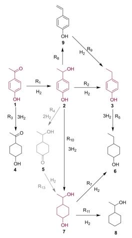
3 Proposed reaction network for the hydrogenation of 4-hydroxyacetophenone, 1, based on species detected in the reaction mixtures. Major reaction species are highlighted.
