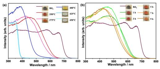
Fig. 5 UV-vis diffuse reflectance spectra of samples thermally treated (a) at temperatures ranging from 350 °C to 450 °C for 1 h and (b) at 350 °C for 1-9 h in air.
