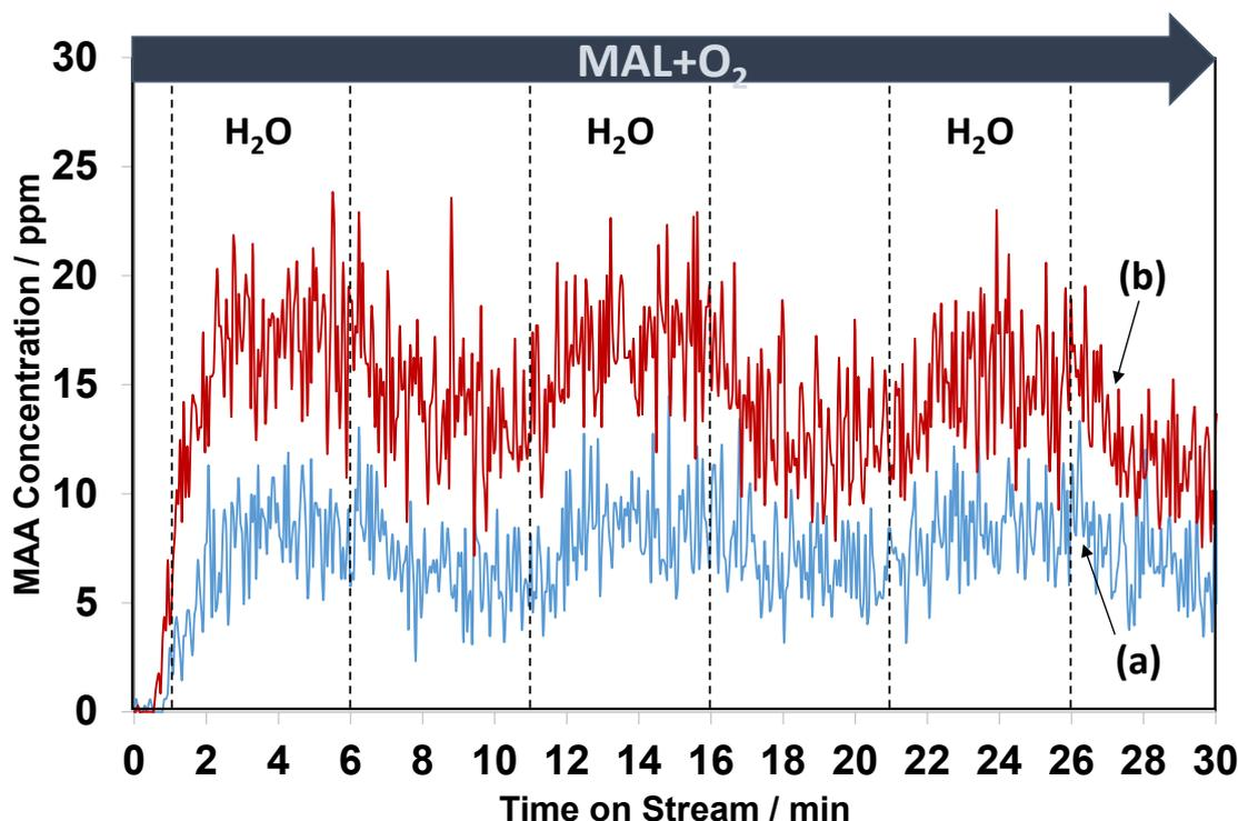
**Figure 6** Changes in gaseous MAA product as a function of time on stream at 320 °C over HPMo (a) and HPMoV (b) samples during the switches of  $\text{H}_2\text{O}$  in and out of  $\text{MAL}+\text{O}_2$  gas feed. Gas feed is composed of 3500 ppm MAL, 7000 ppm  $\text{O}_2$ , 7000 ppm  $\text{H}_2\text{O}$  (when added), and Ar balance and the total flow rate is  $100 \text{ cm}^3 \text{ min}^{-1}$ .
