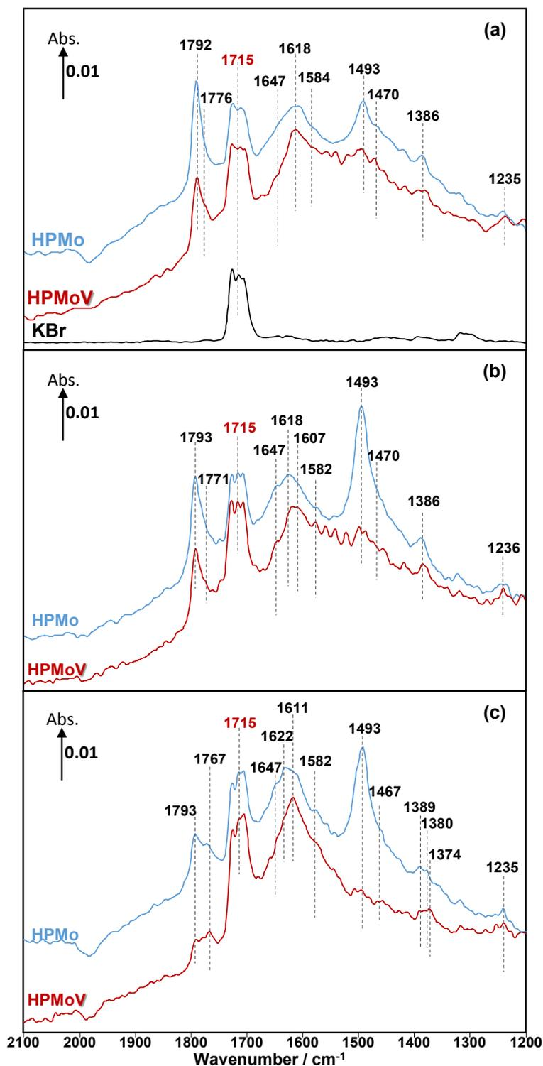
**Figure 2** Comparison of *in-situ* DRIFT spectra recorded at 320 °C over  $\text{H}_3\text{PMoO}_{12}\text{O}_{40}$  and  $\text{H}_4\text{PMoO}_{11}\text{VO}_{40}$  at **2 min** under MAL (a), MAL+O<sub>2</sub> (b), and MAL+O<sub>2</sub>+H<sub>2</sub>O (c). Gas feed is composed of 3500 ppm MAL (when added), 7000 ppm O<sub>2</sub> (when added), 7000 ppm H<sub>2</sub>O (when added), and Ar balance and the total flow rate is 100 cm<sup>3</sup> min<sup>-1</sup>.
