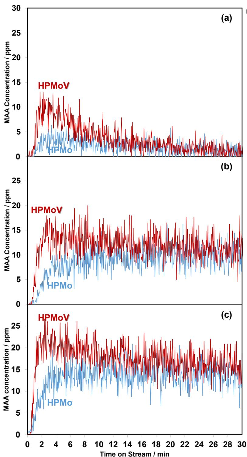
**Figure 1** Comparison of the evolution of MAA formation at 320 °C as a function of time on stream over  $\text{H}_3\text{PMoO}_{12}\text{O}_{40}$  and  $\text{H}_4\text{PMoO}_{11}\text{VO}_{40}$  under MAL (a), MAL+O<sub>2</sub> (b), and MAL+O<sub>2</sub>+H<sub>2</sub>O (c). Gas feed is composed of 3500 ppm MAL (when added), 7000 ppm O<sub>2</sub> (when added), 7000 ppm H<sub>2</sub>O (when added), and Ar balance and the total flow rate is 100 cm<sup>3</sup> min<sup>-1</sup>.
