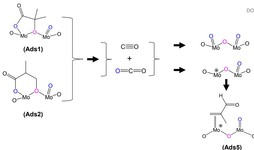
**Figure 5** Proposed formation of by-products CO and CO<sub>2</sub>, derived from lactone-type adsorbed species during MAL adsorption at 320 °C.
