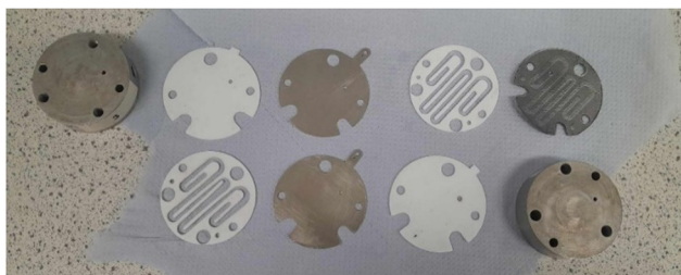
Fig. 2 Electrochemical flow reactor components. 2x stainless steel (SS) electrodes and 1x graphite electrode. 2 PTFE spacers (1 mm thickness) were used, each with a flow channel volume of 0.464 mL. This gave an overall reactor volume of 0.928 mL.
