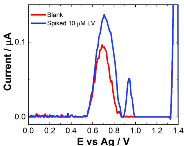
Fig. 7 Typical SWV for neat human pooled serum (red line), and neat human pooled serum spiked with 10  $\mu\text{M}$  LV (blue line) scanned over the potential range  $0 \leq E \leq 1.4$  V vs. Ag at a pulse amplitude of 100 mV and frequency of 40 Hz.
