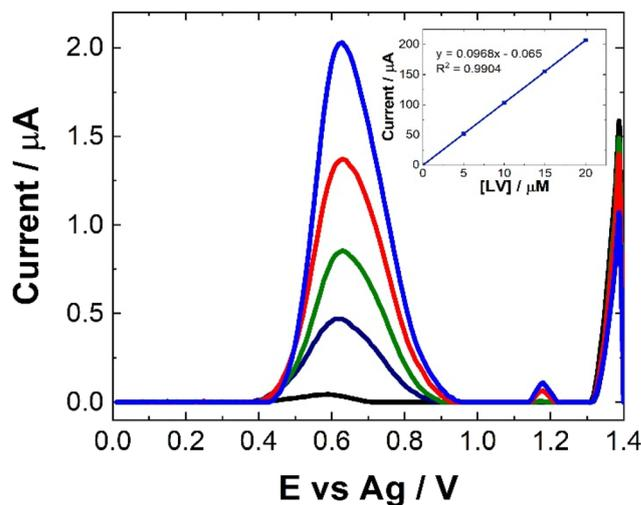
Fig. 8 Typical SWV to increasing [LV] ( $0 \leq [\text{LV}] \leq 20$   $\mu\text{M}$ ) in artificial urine at pH 7 over the concentration range  $0 \leq [\text{LV}] \leq 30$   $\mu\text{M}$  scanned over the potential range  $0 \leq E \leq 1.4$  V vs. Ag at a pulse amplitude of 100 mV and frequency of 40 Hz. Inset shows the typical trend of maximum current at 0.6 V against [LV].
