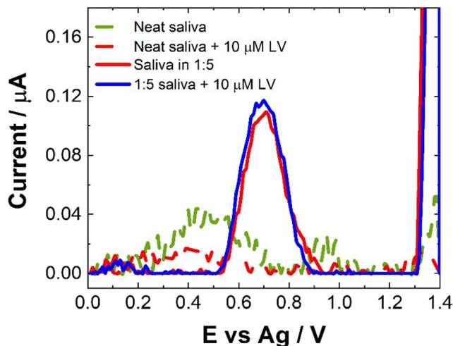
**Fig. 9** Typical SWV for neat saliva (green dashed), neat saliva spiked with 10  $\mu\text{M}$  LV (red dashed); a 1 : 1 dilution of saliva (red line) and 1 : 5 dilution saliva spiked with 10  $\mu\text{M}$  LV (blue line) scanned over the potential range  $0 \leq E \leq 1.4$  V vs. Ag at a pulse amplitude of 100 mV and frequency of 40 Hz. Inset shows the typical trend of maximum current at 0.6 V against [LV].
