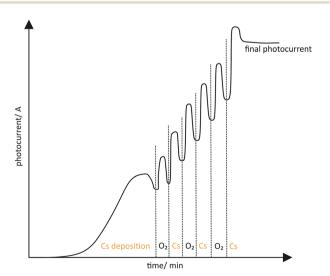
Fig. 9 Schematic drawing of a typical photocurrent evolution when a YoYo activation is used (alternately applying Cs and O2).
