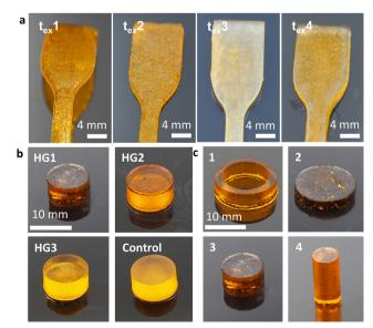
Fig. 2 Overview of the 3D printed hydrogel samples. (a) Comparison of the different exposure times for the optimization of the contour sharpness (5 s; 10 s; 15 s; 30 s), (b) composition, and (c) surface areas.
