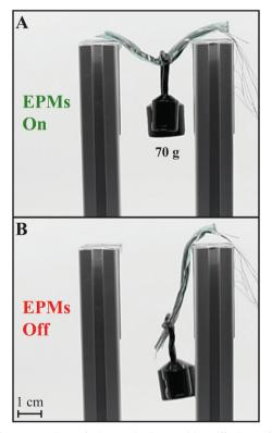
Fig. 11 Demonstration of electronically tunable stiffening of an MRJ beam with fibers scaffolding via EPMs. (A) With EPMs on, the MRJ beam stiffens and is able to hold 70 g of mass. (B) With EPMs off, the MRJ beam resumes its flexible state and can no longer hold 70 g of mass.
