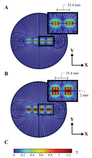
Fig. 4 COMSOL simulations of (A) one row and (B) two rows of neodymium magnets in the 2 mm spacing case with the magnetic field lines in white and xy reference frames. (C) shows the magnetic flux density norm that applies to (A) and (B)
