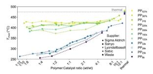
Fig. 5  $T_{\text{max}}$  for cracking of various PP samples obtained from different manufacturers using ECAT at various P: C ratios. For full thermogravimetric analysis (TGA) profiles we refer to Fig. S4 and S5.†
