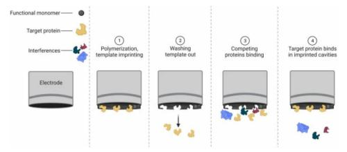
Illustration of BIPs via Electropolymerization. Reproduced from ref. 118 with permission from Elsevier, Copyright 2023
