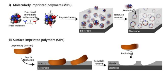
Fig. 2 The approaches used for imprinting: (i) molecularly imprinted polymers (MIPs), (ii) surface imprinted polymers (SIPs). Reproduced from ref. 58 with permission from Elsevier, Copyright 2022.
