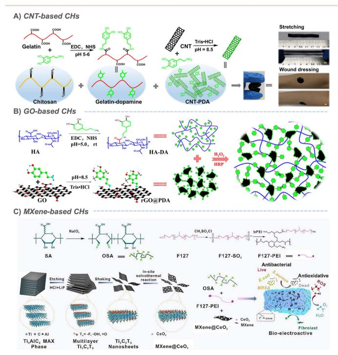
Fig. 2 Carbon-based CHs. (A) CNT-based CHs. Reproduced from ref. 39 with the permission of Elsevier, copyright 2019. (B) Graphene oxide (GO)-based CHs. Reproduced from ref. 40 with the permission of Wiley-VCH, copyright 2019. (C) MXene-based CHs. Reproduced from ref. 57 with the permission of Elsevier, copyright 2021.
