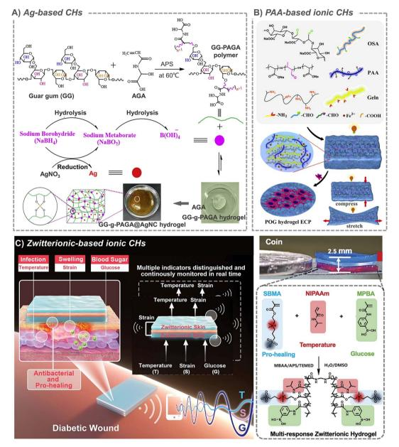
Fig. 4 Metal-based and ionic CHs. (A) Ag-based CHs. Reproduced from ref. 96 with the permission of Elsevier, copyright 2019. (B) PAA-based ionic CHs. Reproduced from ref. 110 with the permission of Elsevier, copyright 2021. (C) Zwitterion-based CHs. Reproduced from ref. 114 with the permission of Wiley-VCH, copyright 2021.
