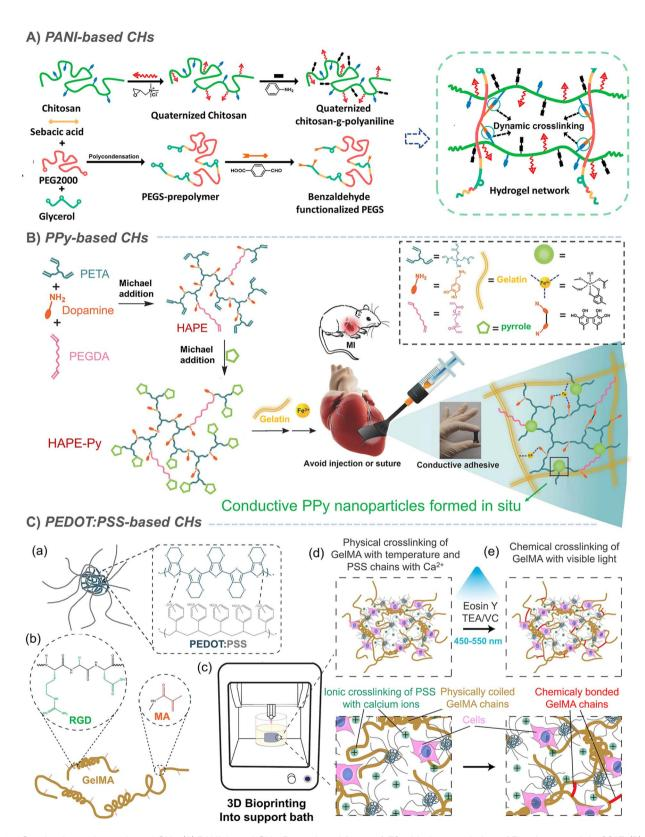
Fig. 3 Conductive-polymer-based CHs. (A) PANI-based CHs. Reproduced from ref. 79 with the permission of Elsevier, copyright 2017. (B) PPybased CHs. Reproduced from ref. 85 with the permission of Wiley-VCH, copyright 2018. (C) PEDOT:PSS-based CHs. Reproduced from ref. 91 with the permission of American Chemical Society, copyright 2019.
