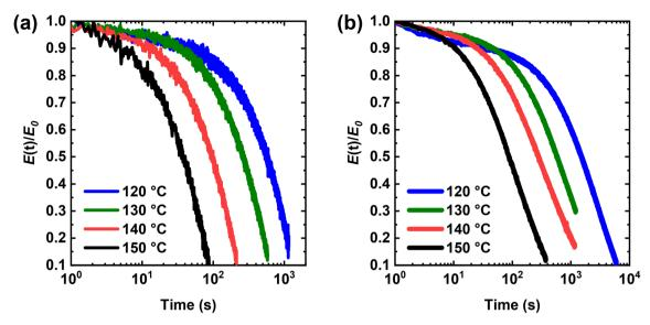
Stress relaxation curves of BiTEBES-based (a) PHMA-5 and (b) PHMA-10 networks at 120-150 °C.
