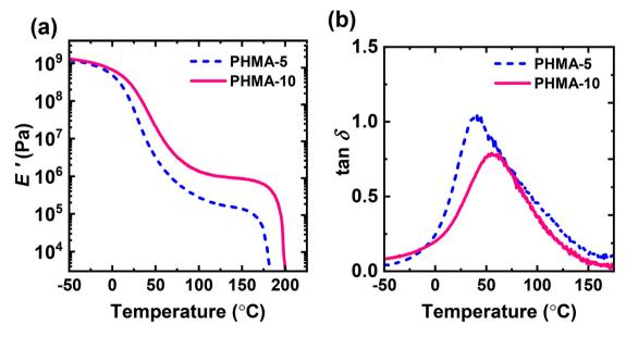
Fig. 5 (a) Tensile storage modulus (E') and (b) damping ratio (tan  $\delta = E''/E'$ ) of BiTEBES-based PHMA-5 and PHMA-10 networks as functions of temperature.
