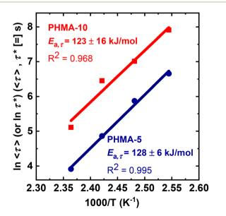
**Fig. 8** Determination of apparent Arrhenius activation energies of stress relaxation for BiTEBES-based PHMA-5 and PHMA-10 networks.
