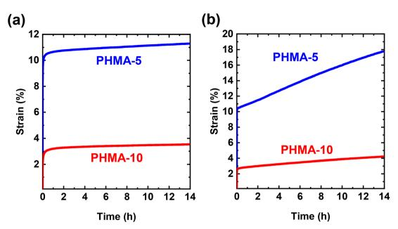
Fig. 9 Creep curves of BiTEBES-based PHMA-5 and PHMA-10 networks at (a) 70 °C and (b) 90 °C.
