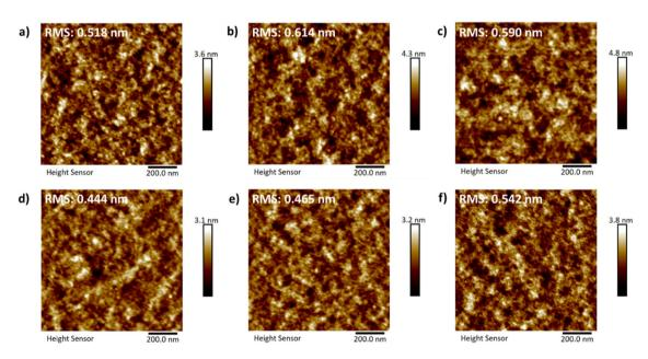
Fig. 3 Atomic force microscopy (AFM) height images with root-mean-square (RMS) surface roughness for *a*-P(iIT)-OH thin films casted from (a) chlorobenzene, (b) *o*-anisole and (c) 20% v/v *o*-anisole/*n*-BuOH; *a*-P(iIT)-TBS thin films casted from (d) chlorobenzene, (e) *o*-anisole and (f) 20% v/v *o*-anisole/*n*-BuOH. Scale bar is 200 nm.
