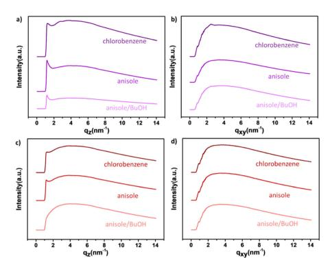
Fig. 2 Grazing-incidence wide-angle X-ray scattering (GIWAXS) scattering profile slices of a-P(iIT)-TBS (a) in-plane and (b) out-of-plane, and a-P (iIT)-OH (c) in-plane and (d) out-of-plane.
