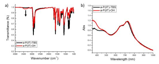
Fig. 1 Fourier-Transform infrared (FTIR) spectra of (a) a-P(iIT)-TBS and a-P(iIT)-OH in the solid-state, and (b) UV-vis spectra of a-P(iIT)-TBS and a-P (iIT)-OH thin films casted on SiO<sub>2</sub>.
