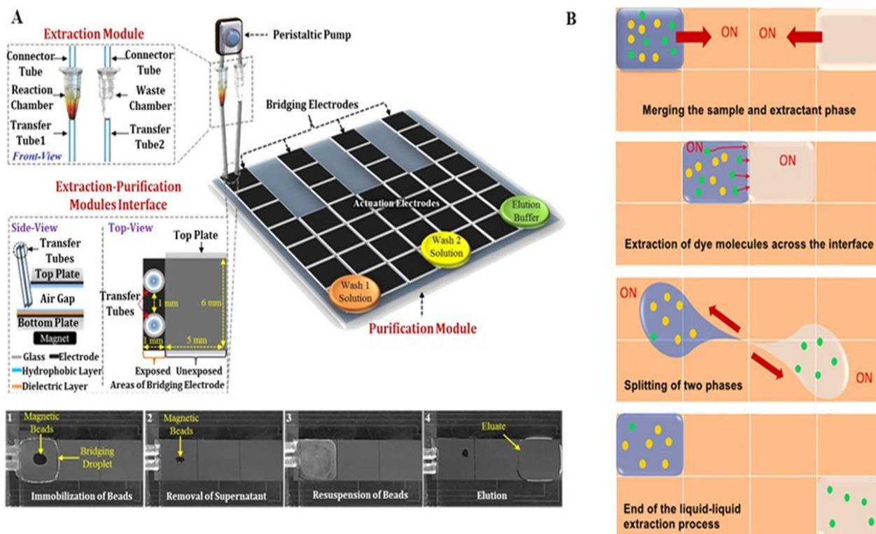
Fig. 7 DMF-based nucleic acid extraction. A) “World-to-DMF” integrated system effectively collecting target analytes based on solid-phase separation. Copyright 2014, the American Chemistry Society.<sup>61</sup> B) Liquid-liquid nucleic acid extraction by handling sample droplets and immiscible extractant phases. Copyright 2021, the American Institute of Physics.<sup>62</sup>
