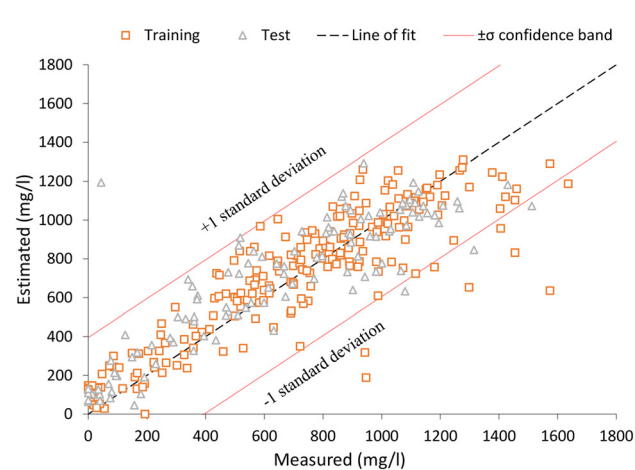
Fig. 5 Scatter plot between laboratory measured COD values (measured) and those estimated by: (A) global model, eqn (6). (B) Individual trend model, eqn (7). (C) Hybrid estimation model. (D) Model based on spectral point values by offspring selection technique, eqn (8).
