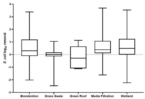
Fig. 1 Log removal of *E. coli* through GSI systems, including bioretention (n = 122), grass swales (n = 39), green roofs (n = 6), media filtration (n = 104), and wetlands (n = 270). Data was accessed from the International Stormwater BMP database on May 1, 2023.
