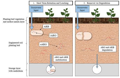
Fig. 2 Potential fates of ARGs and ARB in GSI that captures urban stormwater runoff. 1) The GSI captures and eventually releases ARG and ARB, 2) GSI degrades ARG and ARB, 3) GSI increases the amount of ARB through HGT or selective pressures that enrich ARB.
