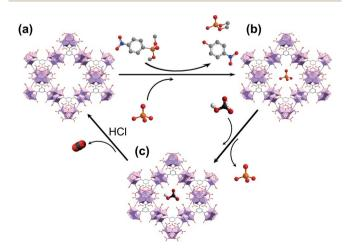
Scheme 1 Schematic representation of (a) simultaneous phosphate removal and pesticide degradation, (b) recovery of phosphate by hydrogen carbonate treatment, and (c) regeneration of MOF-808 with hydrochloric acid.
