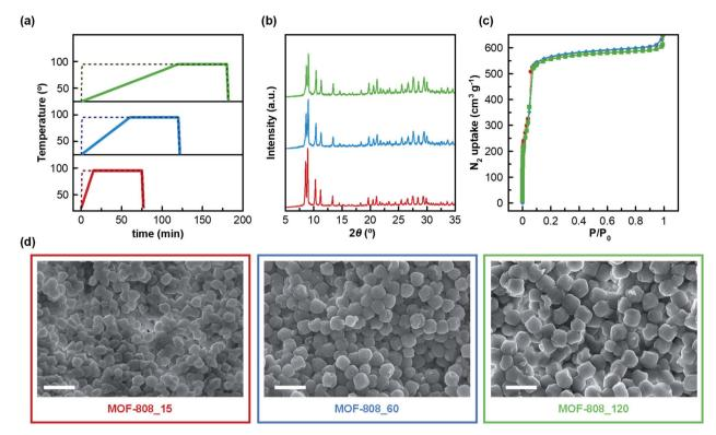
Fig. 1 (a) Controlled-heating ramp used in the preparation of MOF-808 (continuous lines) and control materials (dashed lines). (b) Powder X-ray diffractograms, (c) N2 adsorption at 77 K and (d) SEM images of MOF-808\_15 (red), MOF-808\_60 (blue) and MOF-808\_120 (green). Scale bar: 1 µm.
