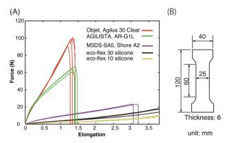
Fig. 2 (A) Results of tensile tests. (B) Overview of specimens used in
