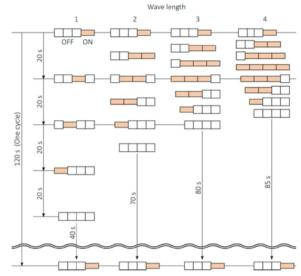
Fig. 10 Four different peristaltic patterns used in the experiments
