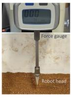
Measurements of burrowing forces of the conical head.
