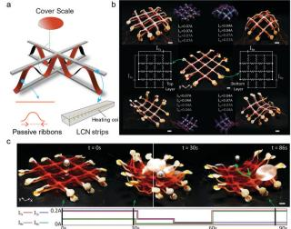
Fig. 5 (a) Illustration of the layered soft robot including the cover scales, heating coil-embedded LCN strips, and passive Kapton ribbons. (b) Different attainable shapes of the robotic surface controlled by four independent current sources. (c) Robotic surface performing different tasks. Reproduced with permission.<sup>74</sup> Copyright 2021, AAAS.
