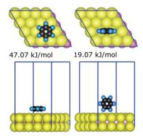
Fig. 1 Top and side views of two benzene-MoS<sub>2</sub> configurations, illustrating the dependence of contact area on binding strength determined from the DFT calculations. Blue lines indicate the periodic cell boundaries.
