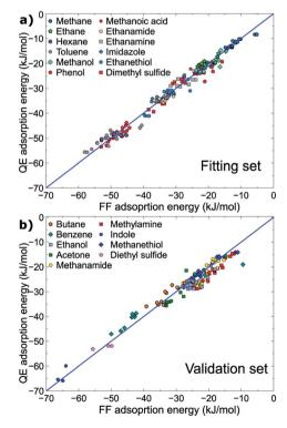
Fig. 2 Correlation between energies produced at the vdW-DF2 level and the MoSu-CHARMM force-field. Data for the (a) fitting and (b) validation sets are plotted separately.
