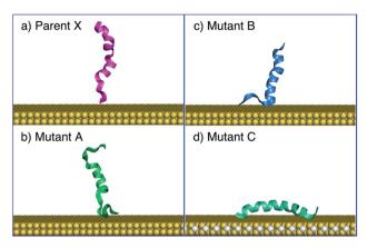
Fig. 4 Side views of predicted adsorption structures illustrating tilting behaviours in panels (a)–(c) of the parent peptide (X), mutant A, and mutant B, whereas mutant C adopted a parallel configuration on  $MoS_2$  and the helicity of its secondary structure was conserved during the simulations, panel (d). Water not shown for clarity.
