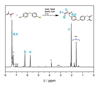
Fig. 2  $^{1}$ H NMR (CDCl<sub>3</sub>) of the crude bifunctional thiomethacrylate crosslinker. Impurity peaks are identified as residual inhibitor p-methoxyphenol (MeHQ, \*), tetrabutyl ammonium bromide (TBAB, \*\*) and toluene (\*\*\*).
