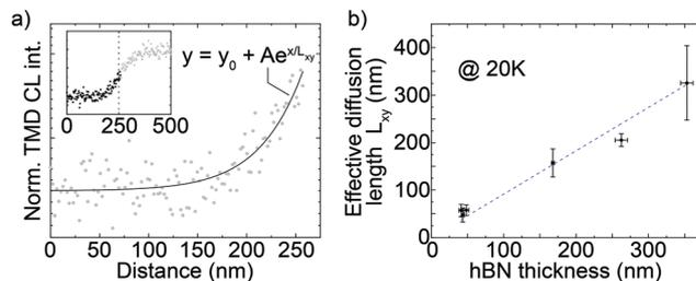
**Fig. 3** (a) Onset of the CL intensity edge response as a function of hBN thickness from Fig. 2c (reported in the inset). The dots are experimental data, the line is the exponential fit to the data according to the equation in the plot. (b) Average values of the effective diffusion length  $L_{xy}$  derived from exponential fit like in (a) as a function of the total hBN thickness. The error bars are the standard deviations of the data.
