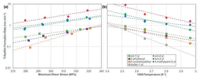
Fig. 5 Change in the tribofilm growth rate for the various ZDDPs with (a) maximum shear stress, τ<sub>max</sub>, at 80 °C and (b) inverse temperature, 1000/ T, at 1000 N (P<sub>max</sub> = 3 GPa). Dashed lines are exponential fits of the data to eqn (1).<sup>13</sup> The rate versus shear stress data for the oct-1-yl and dodec-1-yl ZDDPs at 120 °C are shown in Fig. S5.†
