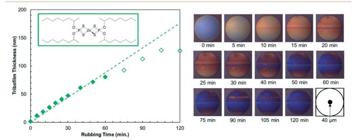
Fig. 2 Representative example (oct-2-yl ZDDP at 80 °C and 1000 N) of the tribofilm thickness growth over time, measured from the SLIM images shown on the right. Dashed linear fits are used to calculate the growth rates (filled symbols only). Black circle (diameter = 40 µm) represents the area over which the mean tribofilm thickness was measured in the central region of the contact.
