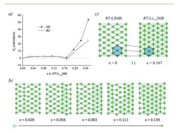
Fig. 6 (a) Energetics of RT-Li<sub>1+x</sub>NiB structure as a function of x. Formation energies are calculated as  $E_F = [E(\text{Li}_{1+y}\text{NiB}) - x \times E(\text{Li}) - E(\text{LiNiB})]/(3 + x)$ , where the  $P2_1/c$  structure is used for x = 0. (b) Top views of the Li layers in the selected optimized structures are plotted. (c) Comparison of Li layer in RT-LiNiB and RT-Li<sub>1+x</sub>NiB.
