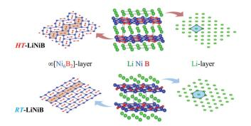
Fig. 1 Crystal structure of RT-LiNiB and HT-LiNiB polymorphs.
