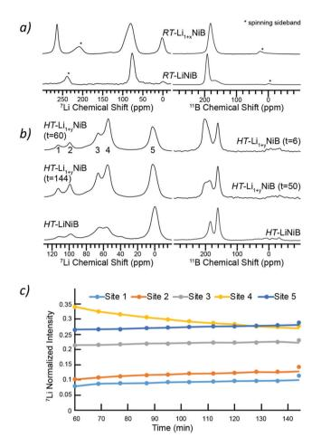
Fig. 11 (a)  $^{7}$ Li and  $^{11}$ B MAS solid-state NMR spectra of RT-Li $_{1+x}$ NiB in comparison to RT-LiNiB phase. (b) <sup>7</sup>Li and <sup>11</sup>B MAS solid-state NMR spectra of HT-Li<sub>1+v</sub>NiB in comparison to HT-LiNiB phase. The time in minutes after starting the magic angle spinning is indicated. (c) Variation in intensities of characteristic peaks (1, 2, 3, 4, 5) with time
