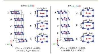
Fig. 4 Comparison between [NiB] layers (ABCB stacking sequence) of RT-LiNiB and RT-Li<sub>1+x</sub>NiB compounds. Bond distances between Ni atoms in the [Ni<sub>6</sub>B<sub>2</sub>] units are highlighted.
