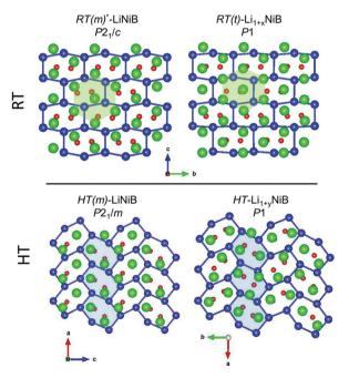
Fig. 8 Comparison of RT-Li<sub>1+x</sub>NiB and HT-Li<sub>1+y</sub>NiB with the RT-LiNiB and HT-LiNiB parents. Light green and blue highlighted areas emphasizes denser packing of Li atoms in the case of RT-Li<sub>1+x</sub>NiB and HT- $Li_{1+\nu}NiB$ , leading to 3 Li atoms per each  $Ni_6B_2$  distorted hexagon.
