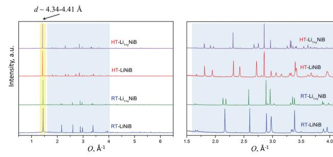
Fig. 3 Experimental synchrotron powder X-ray diffraction patterns of RT-LiNiB [11], HT-LiNiB [11], RT-Li<sub>1+x</sub>NiB and HT-Li<sub>1+y</sub>NiB. The most intense characteristic peak  $d \sim 4.34-4.41$  Å corresponds to the distance between [NiB] layers and is common for all phases. However, compounds have different atomic arrangement within the [NiB] layers, as indicated by the different sequence of the diffraction peaks in the blue-shadowed region, an enlarged view is shown on the right.
