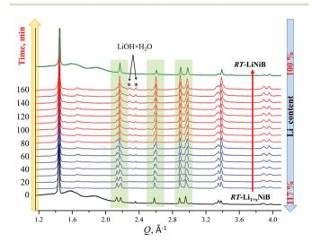
**Fig. 10** X-ray diffraction patterns showing evolution of RT-Li $_{1+x}$ NiB phase (bottom, black) upon expose to air in 0–160 min range. Reference powder pattern of RT-LiNiB compound (top, green) is provided for comparison.
