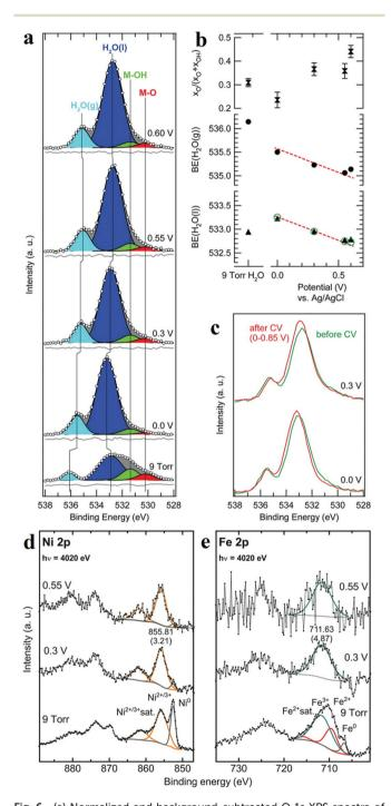
Fig. 6 (a) Normalized and background-subtracted O 1s XPS spectra of Ni-Fe electrocatalyst. (b) Fit results for spectra in (a): relative intensity of the M-O component in the  $MO_x(OH)_v$  catalyst, and measured  $H_2O$  peak positions (black symbols). (c) Comparison of XPS measurements taken at identical applied potentials before (green) and after (red) the second electrochemical conditioning. Normalized XPS spectra of (d) Ni 2p and (e) Fe 2p transitions for a Ni-Fe electrocatalyst. 61
