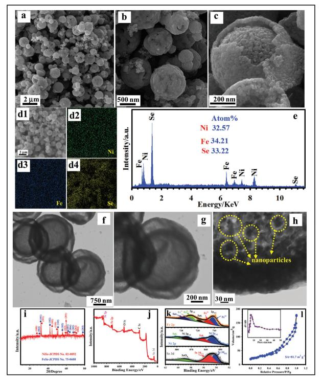
Fig. 4 (a-c) FE-SEM images of DSNFSeHS. (d1-d4) EDS mapping of DSNFSeHS. (e) EDX spectrum of DSNFSeHS. (f-h) TEM images of DSNFSeHS. (i) XRD pattern of DSNFSeHS. (j) Survey spectrum of DSNFSeHS. (k) Ni 2p, Fe 2p, and Se 3d XPS spectra of DSNFSeHS. (l) BET curve of DSNFSeHS and its corresponding BJH plot (inset).
