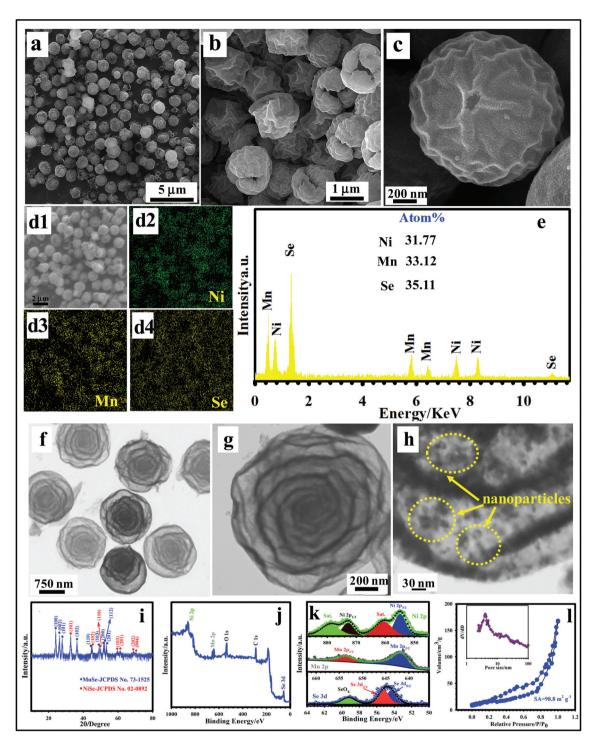
Fig. 2 (a-c) FE-SEM images of MSNMSeHS. (d1-d4) EDS mapping of MSNMSeHS. (e) EDX spectrum of MSNMSeHS. (f-h) TEM images of MSNMSeHS. (i) XRD pattern of MSNMSeHS. (j) Survey spectrum of MSNMSeHS. (k) Ni 2p, Mn 2p, and Se 3d XPS spectra of MSNMSeHS. (l) BET curve of MSNMSeHS and its corresponding BJH plot (inset).
