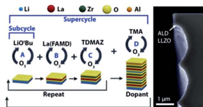
Fig. 6 Schematic representation of an ALD supercycle for the growth of Al-doped LLZO films and the corresponding TEM micrograph. 26
