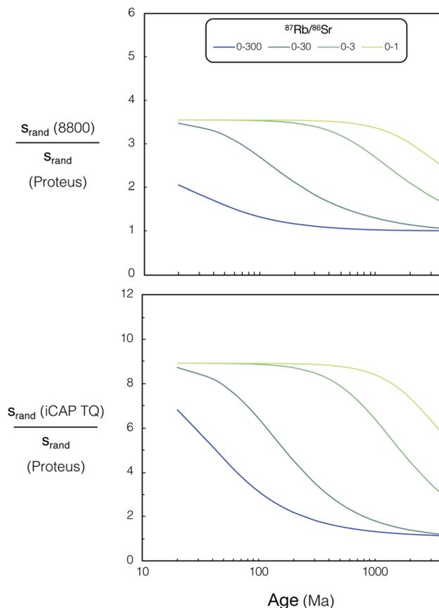
Fig. 13 Relative age uncertainty ratio (Agilent 8800 QQQ)/(Proteus) (top) and (iCAP TQ™)/(Proteus) (bottom) vs. age (20–4000 Ma) for various  $^{87}\text{Rb}/^{86}\text{Sr}$  ranges, see text for details. For tabulated uncertainties and  $^{87}\text{Rb}/^{86}\text{Sr}$  ranges used in this figure please refer to ESI Tables S8 and S9.†
