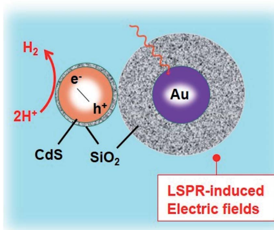
Fig. 4 LSPR-induced electric field immobilized on Au core–SiO 2 . Reproduced with permission from ref. 132.
