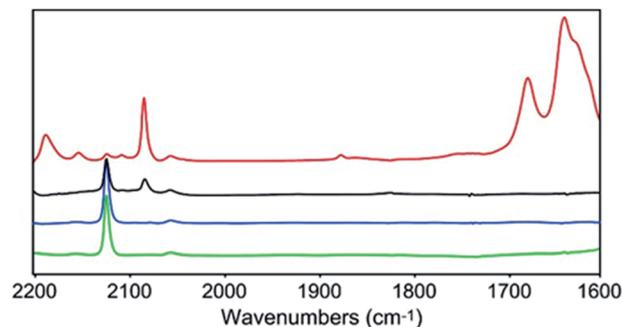
Fig. 4 IR-SEC of complex **1** in dry CH<sub>3</sub>CN with 0.1 M TBAPF<sub>6</sub> at resting potential under Ar (green), CO<sub>2</sub> (blue), and at -2.24(11) V vs. Fc/Fc<sup>+</sup> under Ar (black) and CO<sub>2</sub> (red). LabOMak IR-SEC cell equipped with Pt grid for working and counter electrodes and CE and Ag pseudo-reference electrode.
