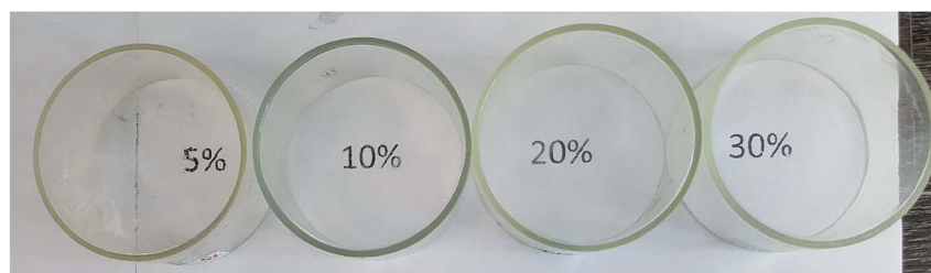
Fig. 30 Photographs of films containing 5, 10, 20, and 30% curing agent, respectively. 141
