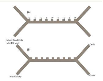
Fig. 2 Microfluidic chip channel (A) location of the voltage input into the microfluidic chip channel (B) input velocities and outputs of blood cells in the microfluidic chip channel.
