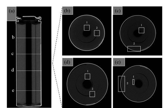
Fig. 2 CT images of retired lithium ion battery: longitudinal section (a) and different cross-sections (b-e). Position 1 and 2 are the weak parts in the battery internal structure.
