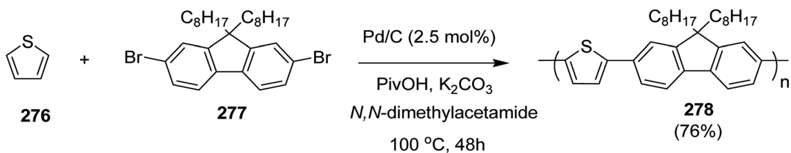
Scheme 80 Direct arylation polycondensation of thiophene using Pd/C to synthesize 278 .
