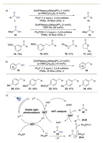
Scheme 3 Deoxygenative reduction of carboxylic acids (a) and benzylic alcohols (b), and proposed mechanism (c).
