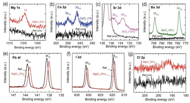
Fig. 5 Mg 1s, Ca 2p, Sr 3d and Ba 3d X-ray photoelectron spectroscopy (XPS) spectra of the annealed FAPbl<sub>3</sub> films with and without additives of (a) MgCl<sub>2</sub>, (b) CaCl<sub>2</sub>, (c) SrCl<sub>2</sub> and (d) BaCl<sub>2</sub>. (e) Pb 4f, (f) I 3d and (g) Cl 2p XPS spectra of the FAPbl<sub>3</sub> films before and after adding the MgCl<sub>2</sub> additive.
