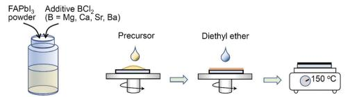
Fig. 1 A schematic illustration of the perovskite deposition procedure. The precursor solution was prepared by mixing the pre-synthesized FAPbl<sub>3</sub> powder with BCl<sub>2</sub> additive (B = Mg, Ca, Sr and Ba), which was spin-coated. Diethyl ether was dipped for 20 s after rotating the substrate. The film was annealed at 150 °C in an air atmosphere
