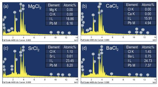
Fig. 4 Energy dispersive X-ray spectroscopy (EDS) of FAPbl<sub>3</sub> films with additive of (a) MgCl<sub>2</sub> (5%), (b) CaCl<sub>2</sub> (1%), (c) SrCl<sub>2</sub> (10%) and (d) BaCl<sub>2</sub> (9%).
