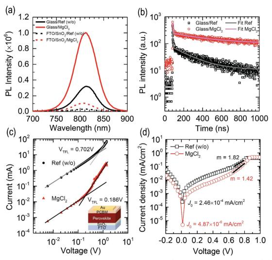
Fig. 7 (a) Steady-state photoluminescence (PL) of the FAPbI<sub>3</sub> film with and without MgCl<sub>2</sub> deposited on a glass substrate and SnO<sub>2</sub>-coated FTO substrate. (b) Time-resolved PL (TRPL) for the FAPbl<sub>3</sub> film with and without MgCl<sub>2</sub> on a glass substrate. Dark current density (J)-voltage (V) curves for (c) the FTO/SnO<sub>2</sub>/FAPbI<sub>3</sub> (with or without MgCl<sub>2</sub>)/PCBM/Au electron-only device and (d) the full solar cell device.
