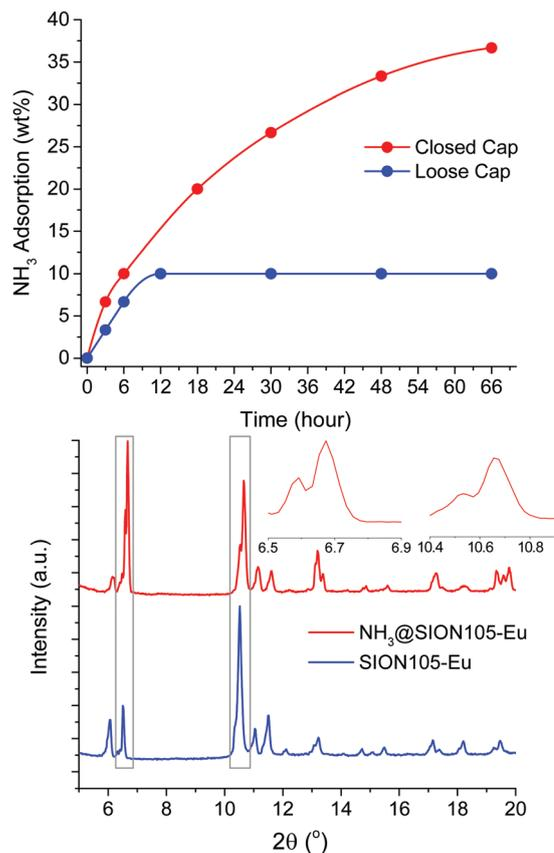
Fig. 2 (top)  $NH_3$  adsorption curve for **SION105-Eu** as a function of time; (bottom) PXRD pattern of the **SION105-Eu** sample after 6 hour of  $NH_3$  vapour adsorption in comparison to the as-made sample. Inset: The appearance of new peaks within the selected regions.
