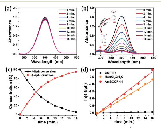
Fig. 5 Catalytic reduction of 4-nitrophenol by using NaBH<sub>4</sub>, (a) COPN-1, (b) with Au@COPN-1 ( $4.6 \times 10^{-3}$  mM Au), (c) kinetics of reduction process of 4-Nph solution (4-Aph formation) and (d) fitted data of the pseudo-first-order kinetics (Au@COPN-1, HAuCl<sub>4</sub>·3H<sub>2</sub>O, and COPN-1).
