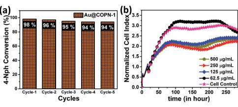
Fig. 6 (a) Recycling experiment of Au@COPN-1 for the conversion of 4-Nph during 5 cycles of reaction and (b) real-time cell analysis results: effect of Au@COPN-1 treatments on L929 cell line proliferation.
