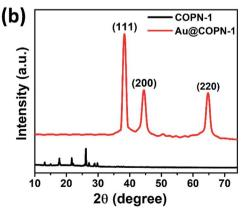
Fig. 2 (a) UV spectra and (b) XRD Pattern of COPN-1 and Au@COPN-1  $(4.6 \times 10^{-3} \text{ mM Au})$
