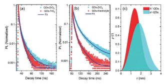
Fig. 4 Comparison of the transient PL curves of heterostructured QDs: (a) deposited onto a ZrO2 and TiO2 mesoporous film; (b) deposited onto a ZrO2 mesoporous film and QDs with electrolyte. The excitation wavelength is  $\lambda_{ex}$  = 444 nm. (c) Comparison of the spatial probability distribution value  $\rho(r)$  of the electron and hole as a function of QD radius r (nm) (H = 2.15 nm, red for hole and cyan for an electron).
