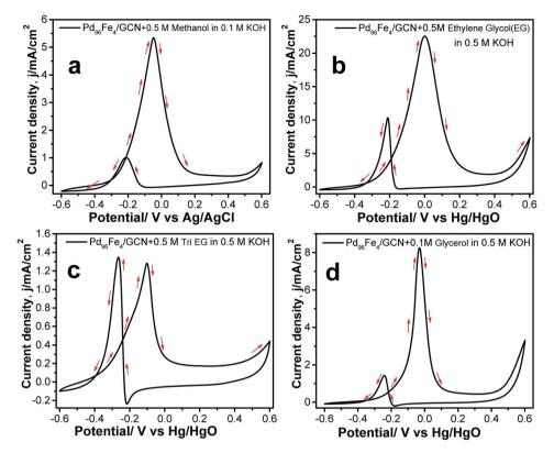
Fig. 8 CVs for the electrocatalytic oxidation of (a) 0.5 M methanol in 0.1 M KOH, (b) 0.5 M ethylene glycol, (c) 0.5 M tri-ethylene glycol, and (d)  $0.5~{\rm M}$  glycerol at the  $100^{\rm th}$  cycle by  ${\rm Pd_{96}Fe_4/GCN}$  in  $0.5~{\rm M}$  KOH at a scan rate of  $50~{\rm mV}~{\rm s}^{-1}$
